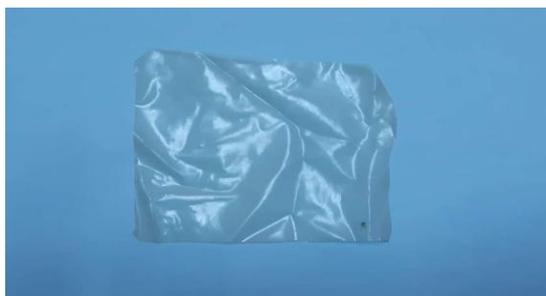
Figure (4) Bioplastic Film Using Dent Corn Starch
