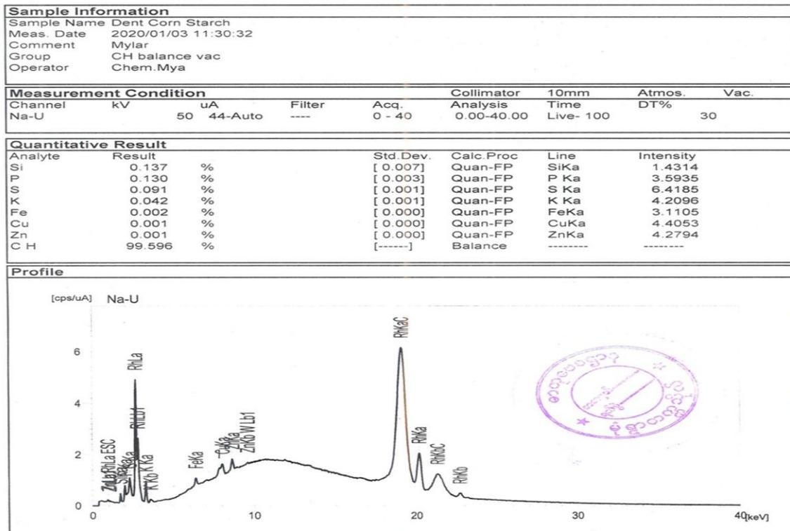
Figure (3) EDXRF Spectrum of Prepared Dent Corn Starch
